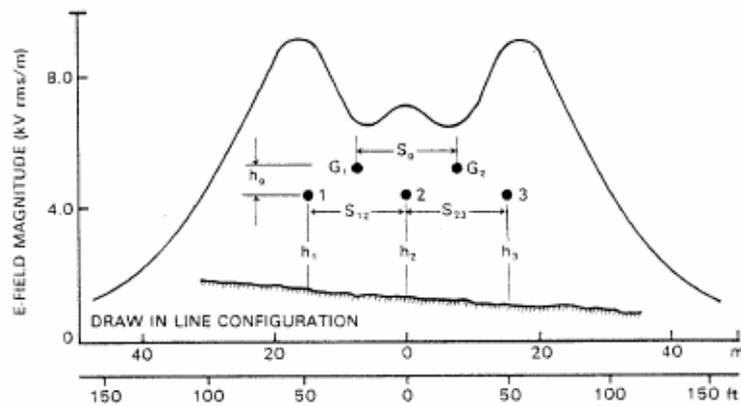
NOTE—The symbols ( $h_1$ ,  $S_{12}$ , etc.) represent conductor heights and spacings.
